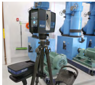
With FARO’s laser scanners and software, one person can “capture in a few hours what a team of people used to do over the course of a week,” said Mark Lamberson CPD, National Virtual Design and Construction Manager for Limbach Holdings Inc.
