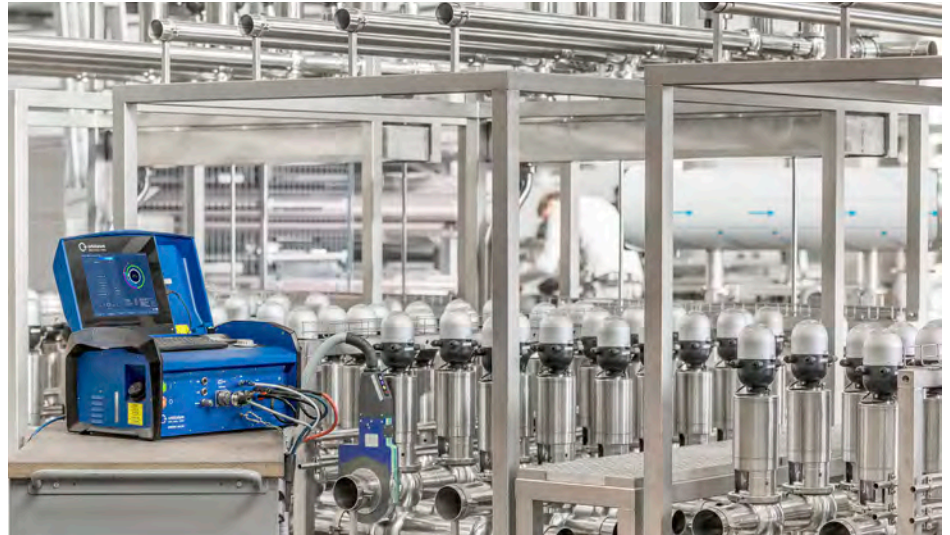
HPS found that Orbitalum's OM 180 SmartWelder's standard Flow Force, a purge gas function, dramatically shortened welding cycles as they worked to rapidly expand infrastructure for COVID-19 vaccine research and production.
