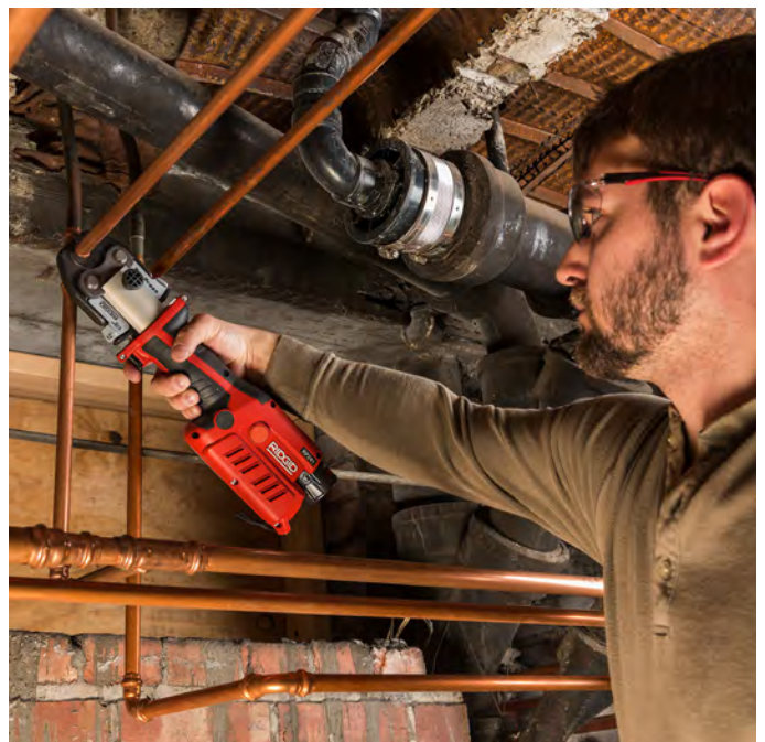
RIDGID's RP 241 compact press tool connects to your phone via Bluetooth, so you can easily keep track of the battery life and cycle counts, avoiding unexpected maintenance on the jobsite.
