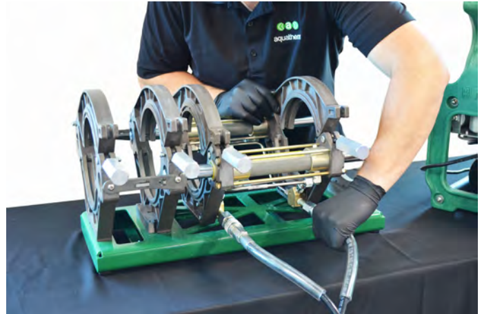
Preparing the fusion machine will help ensure that you can perform effective butt fusion of polypropylene piping, which creates leak-free joints.
