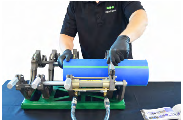
Clamps hold the pipe as it is being fused, and an accurate alignment will ensure a consistent fusion bead, which is important for a good connection.
