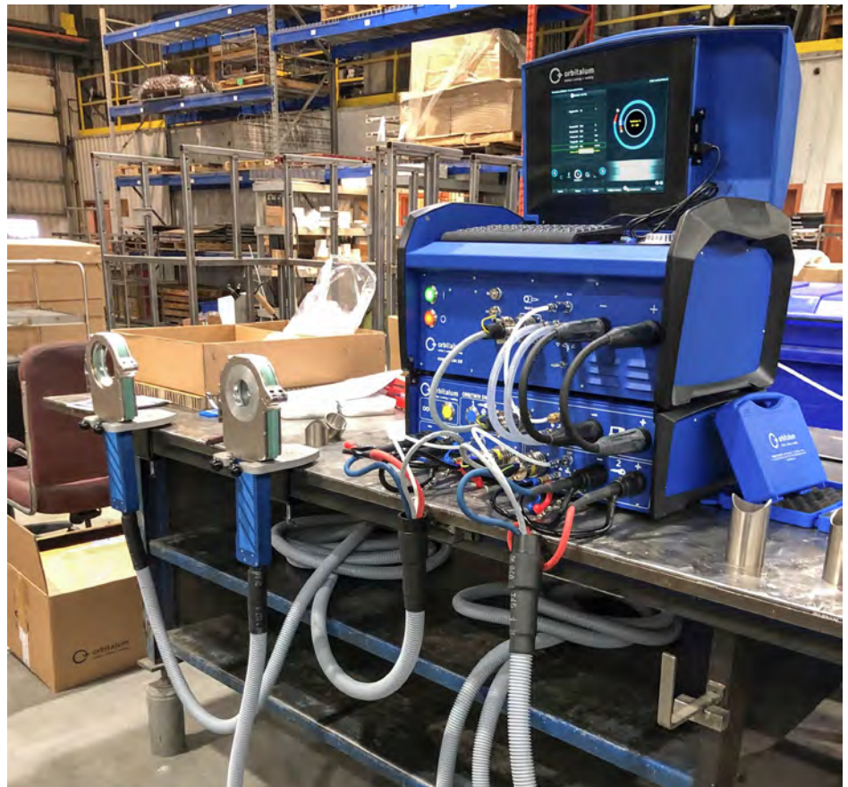
HPS combined Orbitalum's OM180 SmartWelder TIG orbital welding power supply and fully enclosed, water-cooled weld heads with the Orbitwin SW switching unit, which offers the flexibility to control two orbital welding heads with one power supply, providing HPS a huge productivity increase.
