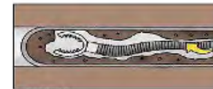
Opening with cable
