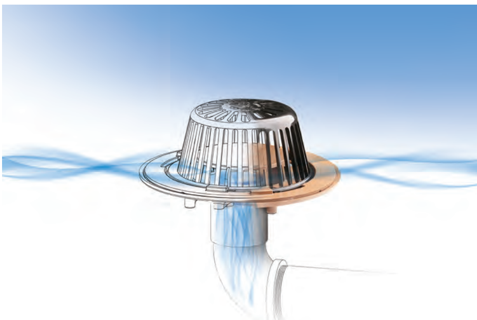
Smith siphonic drains, combined with a properly designed siphonic system, will completely fill up, or prime, with water and initiate a siphonic flow within as little as 15 seconds.
