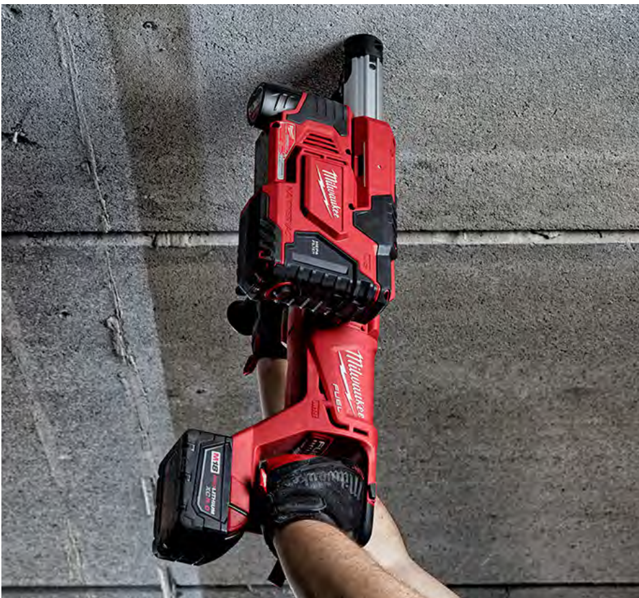
McGilvray Mechanical made a seamless transition to compliance with new OSHA standards protecting workers from respirable silica by using MILWAUKEE's HAMMERVAC™ Dedicated Dust Extractors in conjunction with their current M18 FUEL™ 1-1/8" SDS Plus Rotary Hammers.
