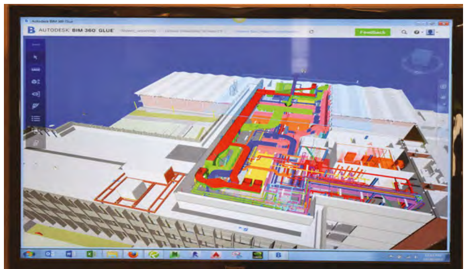
Arden Engineering Constructors relies on Trimble's TX6 Scanner to capture a building's MEP details much faster and more accurately than workers measuring by hand. Using RealWorks software in concert with their other BIM programs, they translate the data into digital models that are essential to effective planning and coordination among all the contractors involved.
