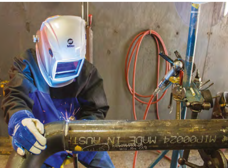
Advanced welding processes such as pulsed MIG and RMD offer consistent weld quality and increased productivity thanks to travel speeds that are three to four times those of stick or TIG.
