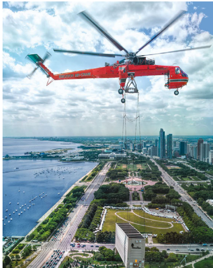
Using Erickson's precision capabilities and the lift capacity of the Aircrane helicopter, aerial crane operators placed chiller equipment on the roof of a downtown Chicago building, cutting the Hill Group's installation time to hours compared with weeks needed for other methods.
