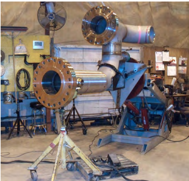
The Team Industries positioner includes steel-hardened insert jaws with small-bore adapters to eliminate the need for modified C-clamps.
