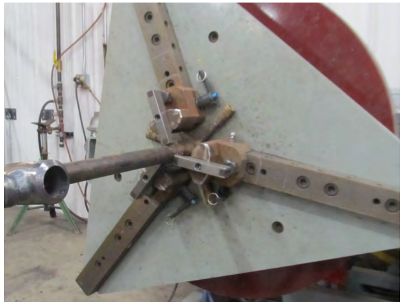
The Team Industries positioner includes steel-hardened insert jaws with small-bore adapters to eliminate the need for modified C-clamps.
