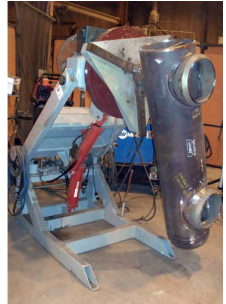
Team Industries' weld positioner accommodates an eccentric load rotated to allow high deposition weld processes.
