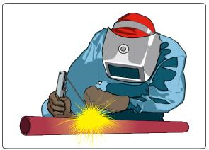
Welding, cutting and heating are methods of melting, cutting or heating metal with electrical current or compressed gases. The biggest concerns with welding, cutting and heating in mechanical fabrication shops are electrical shock from electric arc welding, eye hazards, fire hazards and respiratory hazards.
