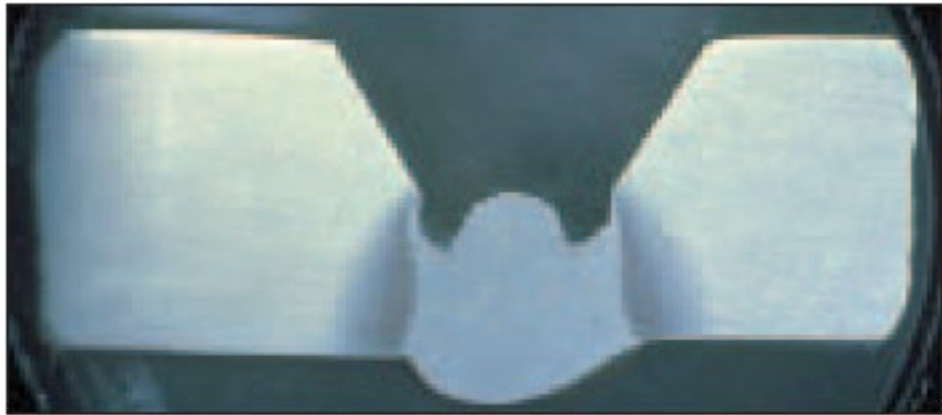
Open Root Pass with Stick Electrode
