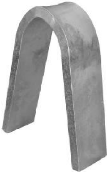
Figure 1: In a bend test, a flat strap of metal is bent into a U-shape, stretching the material on the outer surface of the "U," while compressing the material on the inside surface.
