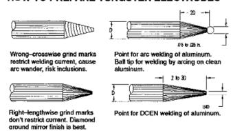
Regardless of the electrode tip geometry selected, it is important that consistent electrode geometry be used once a welding procedure is established. Changes in electrode geometry can significantly influence the weld bead shape and size; therefore, electrode tip configuration is a welding variable that should be studied during the welding procedure development.
