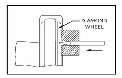
Before regrinding, a used electrode is reconditioned by diamond grinding a new fiat at the tip.
