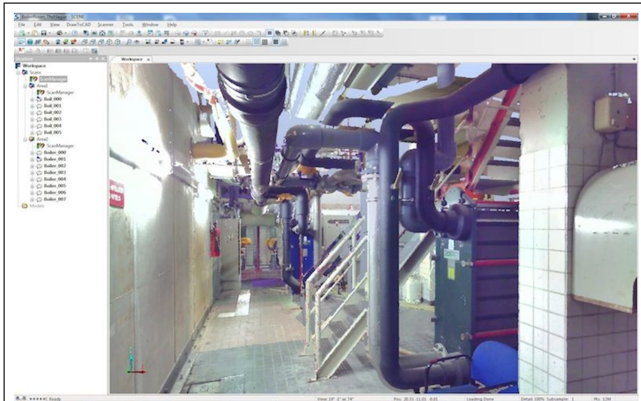
FARO Scene showing a scan. The photosphere is shown in the navigator, and measurements can be made by clicking any two points (image by SPAR Point Group).
