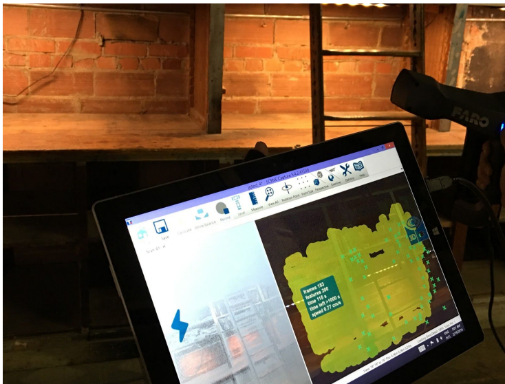
The SCENE Capture app running on a Microsoft Surface Pro tablet powers the FARO Freestyle and processes the scan as it is captured by the sensor.
