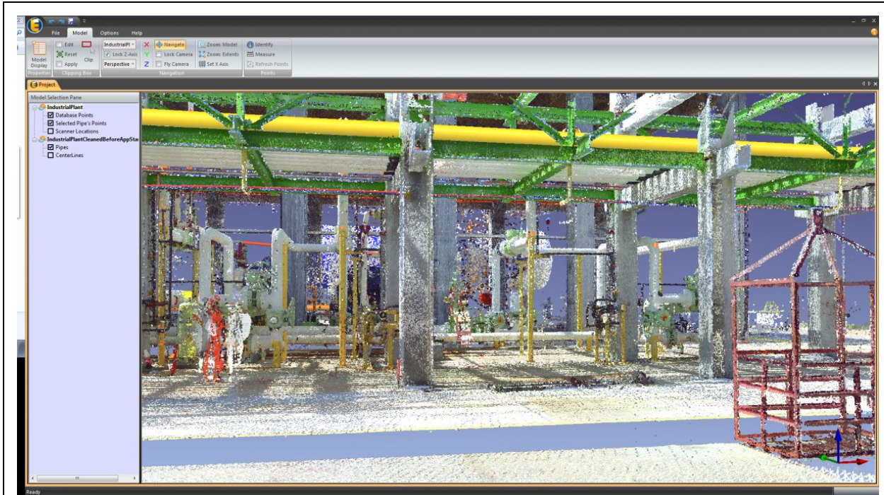
Structural steel and piping generated from the point cloud (image by Trimble).
