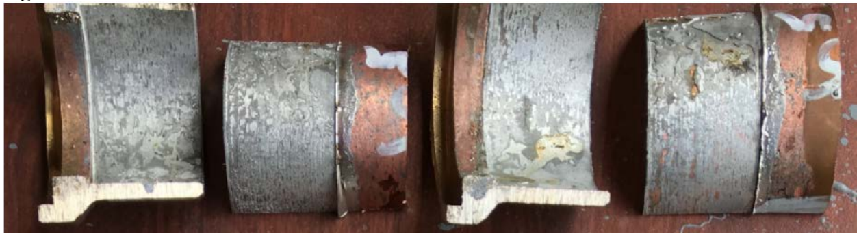
Faying surfaces exhibit lots of incomplete fill on one side due to non-uniform heating. Figure 4
