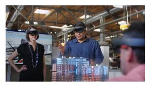
There is a slight difference in the visual you will see in live stream mode. While wearing the device, you have a limited range of visualization of the model that can be displayed of about 30 x 17.5 degrees. When live streamed through a PC, the entire model, including the portion outside of the users' field of view is visualized on screen.
