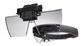
get the proper angle, there is a tilt mechanism that allows the user to slightly tilt the wave guide to find the proper angle.
