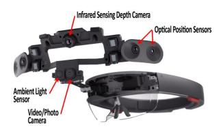
information. The optical position cameras are used to constantly determine where the device is within that space in order for the holograms to appear to not move. The ambient light sensor is used to determine brightness level of the projections and the front facing video/photo camera is used to take pictures and videos with the unit.
