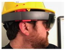
• <u>Glasses</u> – If a user has prescription glasses, they need to be worn underneath the HoloLens device in order to clearly see the holographic visualizations. If the user has large glasses or they sit on a similar position on the nose as the HoloLens nosepiece, this can be uncomfortable or prevent the user from experiencing the visualization.
