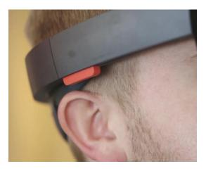
The device does not allow for audio input from headphones. It requires any audio input to come from the microphone array incorporated in the device. Four noise-cancelling microphones are included in this array between the orange speakers and the optical sensors. They provide excellent sound quality.
