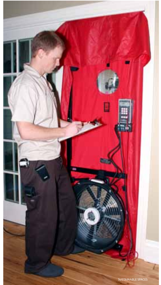
A technician from Sustainable Spaces, a home performance contractor based in San Francisco, conducts a blower door test to identify air infiltration.
